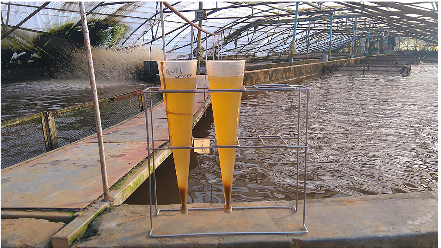
Figure 1. Imhoff cones are used to measure biofloc volume in BFT tanks at Chambo Fisheries.
