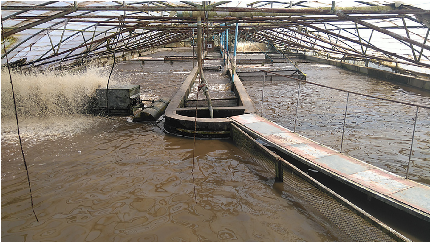
Figure 5. A single multi-cohort sequential 766-m3 SAFF-BFT grow-out tank at Chambo Fisheries.
